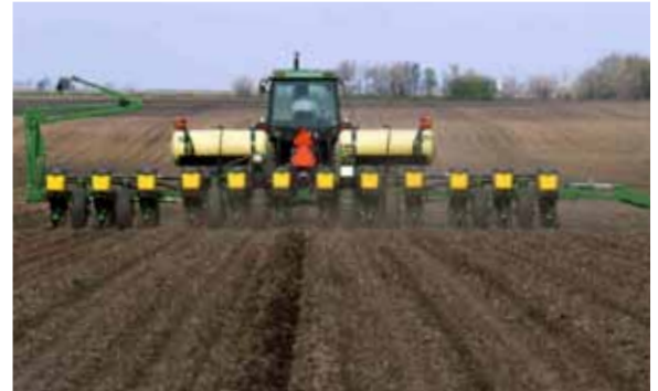
One way to help ensure that proper seeding depth is maintained across a field is to operate the planter at the proper speed.
